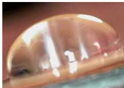
Silicone paper: Surface tension: < 30 \text{ N/mm} . Very poor surface wetting. Very hard to stick for this reason.
