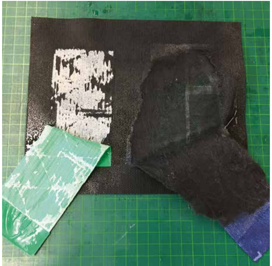
Adhesive tape after storage in water for 24 hours: Top: a conventional acrylate dispersion adhesive tape, re-emulsified with water; the adhesive has lost its strength. Bottom: pure acrylate on a solid basis is absolutely water-resistant.
