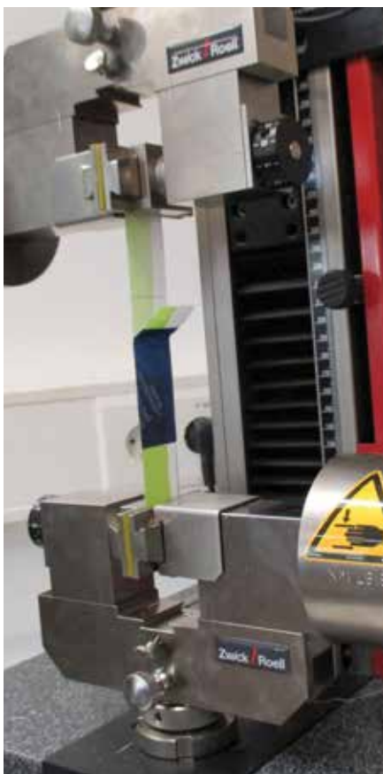
The forthcoming standard DIN 4108-11 will specify laboratory tests that have to be carried out for all adhesive tapes. This will create consistent quality standards and provide a basis for users to compare products.
