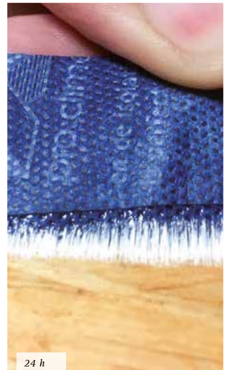
These photos show how strength builds up over the course of contact time. An adhesive tape was employed here that can be used for interior air sealing and exterior wind sealing. The initial adhesion – after 20 minutes – can be seen on the left; the significantly stronger adhesive bond after 24 hours can be seen on the right.
