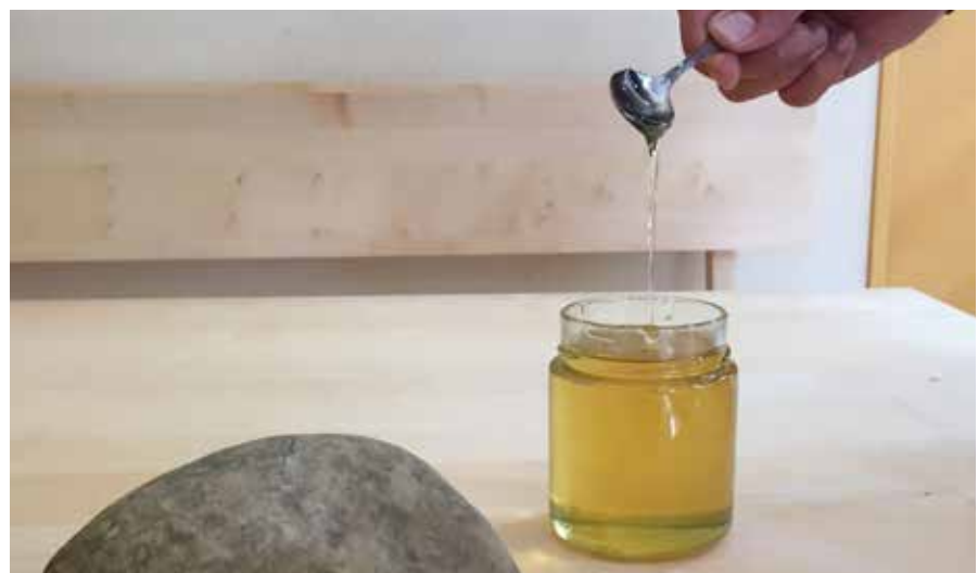
Honey has high adhesion – it sticks immediately to every surface. However, its cohesion is low, which means that honey drops off the surface under the action of its own weight. Stone is the exact opposite: it has high inner strength, i.e. cohesion, but has no adhesion and therefore does not stick to surfaces.
